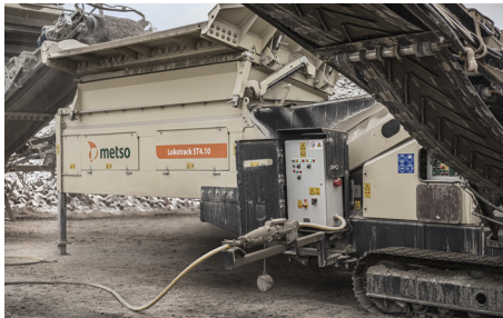
e-Power for efficient hybrid diesel-electric operation.
